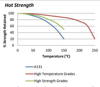
to ISO 10964. Cured at 23°C for 24 hours then conditioned for 30 minutes at testing temperature.
