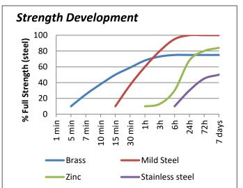
Permabond activator A905 or ASC10. Alternatively, increasing the curing temperature will reduce curing time.
